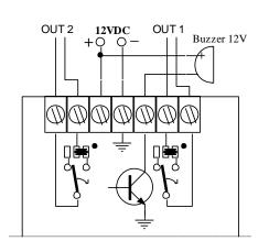
Installation schematic diagram of the DW200HM miniature receiver:
