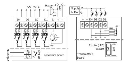
The RP501 transmitter may be either powered by 12VDC supply screwed to +/- connectors or, by 3V (2x AA) battery or, by both power sources simultaneously.
