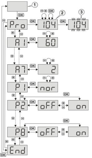
At standby LED is off. Enter programming procedures by pressing OK. Select programming parameter with + and - buttons. To exit procedure select End on display and press OK, or wait 16s.
