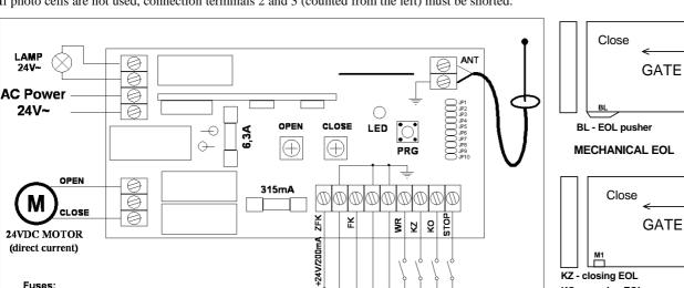
If photo cells are not used, connection terminals 2 and 3 (counted from the left) must be shorted.
