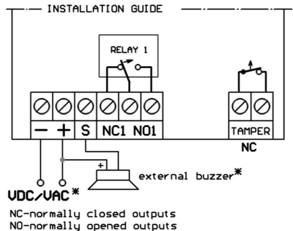
**IMPORTANT! Output S must not** be directly connected to (+) pole of power supply (see schema).
